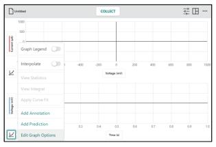
Modify the x- and y-axis ranges to replicate the waveform graph determined by the CV profile.
