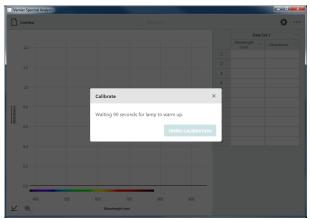
3. When the lamp warm up is complete, place a blank cuvette in the holder with the clear sides aligned with the arrow on the spectrometer. Click or tap complete the calibration.
