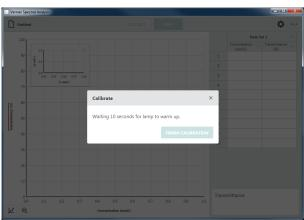
3. When the lamp warm up is complete, place a blank cuvette in the holder with the clear sides aligned with the arrow on the spectrometer. Click or tap FINISH CALIBRATION to complete the calibration.
