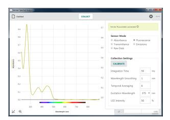
7. Adjust the Excitation Wavelength to select the wavelength you want to use. The wavelength options shown depend on the spectrometer you are using.
