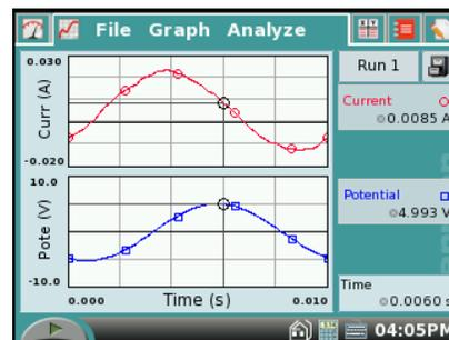
The calculations using the component values would predict that the current would lead the voltage by  $70$  degrees and the result matches this well.
