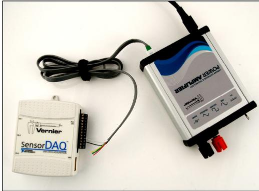
SensorDAQ is a lab interface for use with LabVIEW and engineering education. The analog output on SensorDAQ is on the screw terminal connections. It has a 0 to 5 volt output. There are two ways to make the connection from SensorDAQ to the Power Amplifier:
