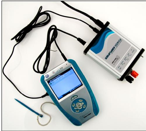
Connect the output of the Power Amplifier across a device such as a light bulb or resistor. Use Logger *Pro* or LabQuest App to plot the current through the component versus the potential across it. It is particularly interesting to compare a light bulb to a resistor.
