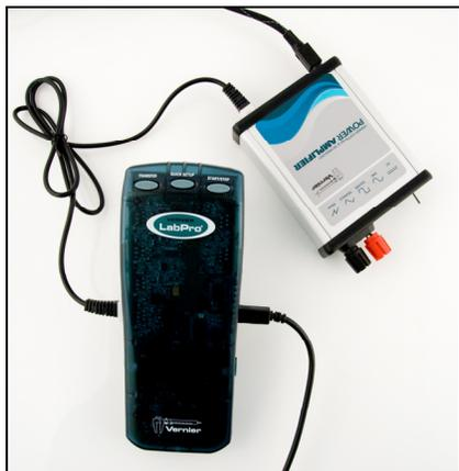
*Power Amplifier connected via the BTA cable to CH 4 of a LabPro*
