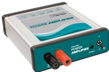
The Vernier Power Amplifier allows you to drive loads with  $\pm 10$  V and currents up to 1 A. It works with any input waveform, including DC, sine, square, triangle, and sawtooth waveforms. The Power Amplifier can drive a variety of loads, such as speakers, lamps, small DC motors, and RLC circuits. These circuits typically draw more power than the signal source can deliver. The Power Amplifier makes it possible to drive these heavy loads.
