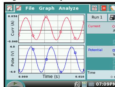
The current and voltage graphs below were made with an RLC circuit with a  $0.067 \text{ H}$  inductor, a  $4.7 \mu\text{F}$  capacitor, and a  $100 \Omega$  resistor.
