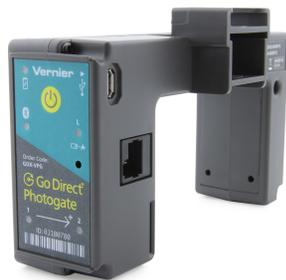
Go Direct Photogate is used for velocity, acceleration, and timing measurements of objects passing through the gate. The object blocks infrared beams as it passes through the gate. Motion data can be determined from the timing of beam blocking.
