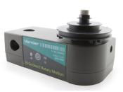
Go Direct Rotary Motion is a bidirectional angle sensor designed to measure rotational or linear position, velocity and acceleration. It is used for a variety of applications, including
