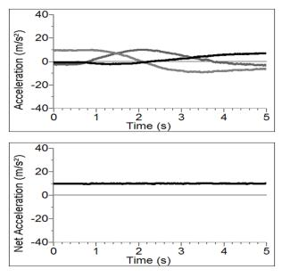
Rotating the 3-Axis Accelerometer
