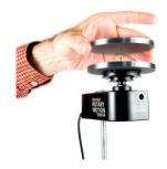
Motion of a Physical Pendulum (requires Rotational Motion Accessory Kit, see Accessories section)
