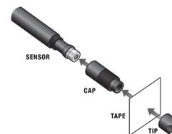
Figure 1 Assembly of sensor, cap, tape, and tip
