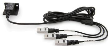
The 3-Axis Accelerometer consists of three  $-5$  to  $+5$  g accelerometers mounted in one small block. Using the appropriate data-collection hardware and software, you can graph any of these components, or calculate the magnitude of the net acceleration. The 3-Axis Accelerometer can be used for a wide variety of experiments and demonstrations, both inside and outside the lab.
